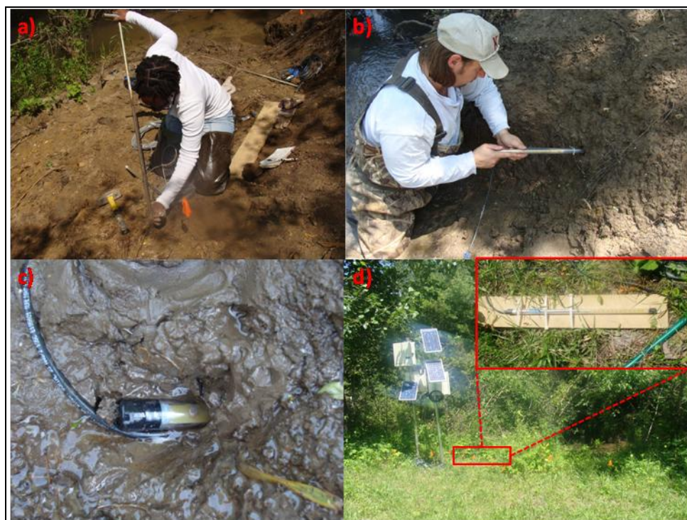
Figure 3.13: Installation procedure for the PEEPs.
